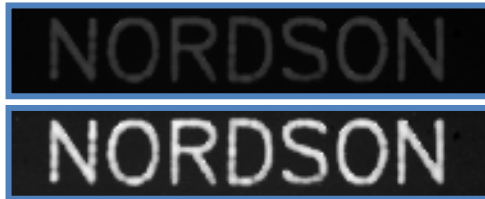
Example of Software Programmable Camera Gain Adjustment
