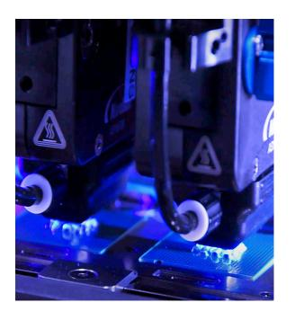
Simultaneous dual-valve dispensing with the IntelliJet Jetting System improves yield and reduces production costs.
