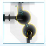
Easily ensure IPC compliance with automatic measurement and voiding analysis that gives clear pass/fail results.
