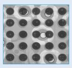
Voiding in a Micro BGA array.
