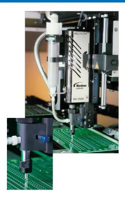
The DV-7000 Heli-Flow Pump is available in a lueror footed-needle design with interchangeable cartridges, allowing each pump to work with several different fluid types. The DV-7000 has a hardened auger for use with filled epoxy materials and features a high flow rate.
