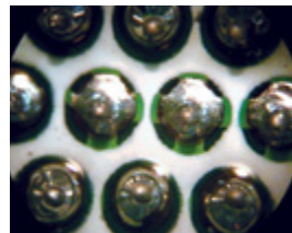
Solder paste and preforms reflowed
